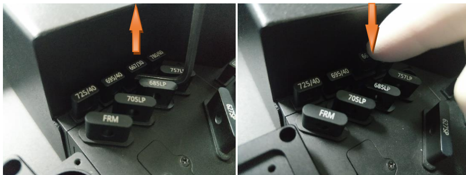
Figure 29. Change the Optical Filter or Dichroic Mirror
