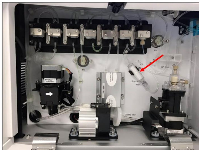
Figure 97. Location of Sheath Fluid In-line Filter
