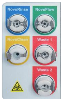
Figure 25. Interface of the Fluidics Ports
