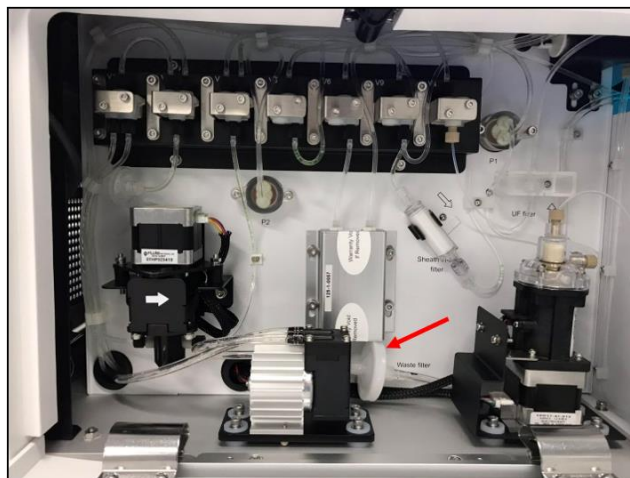
Figure 98. Location of Waste Filter
