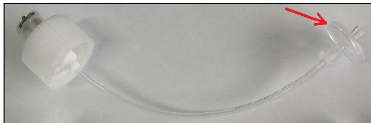
Figure 101. NovoRinse and NovoClean Solution Inlet Filter
